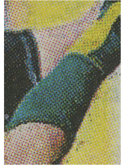
Figure 3.3: Magnified newspaper, showing that an image is made up of dots of coloured ink
