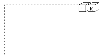
(b) The representation of a colour image in OpenCV and numpy, a 2D array of 1D pixels
