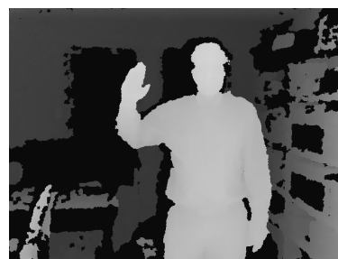
Figure 1.8: A depth image captured from a Microsoft Kinect, with brighter meaning closer to the camera.
