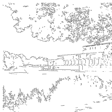
(b) Edges obtained using Canny's detector
