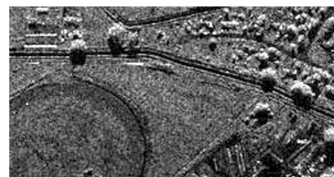
Figure 1.7: A synthetic aperture radar (SAR) image. Note how noisy it is compared to a conventional image, a combination of the need for the radar to illuminate the scene and the coherent nature of the imaging.
