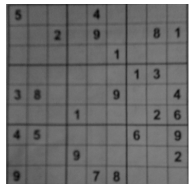
Figure 1.15: The image after rectification to a rectangle
