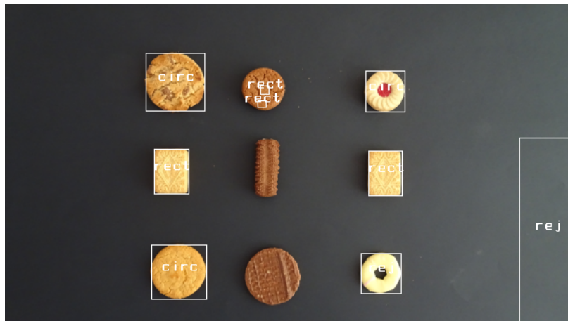
Figure 5.8: Identification of circular and rectangular biscuits. Note that there is a spurious region due to uneven illumination and how difficult the brown biscuits have been to distinguish from the background
