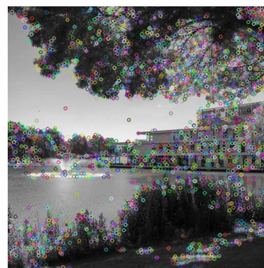
Figure 7.15: SIFT features marked on a natural image
