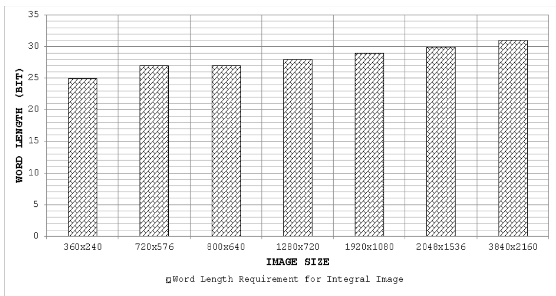
Figure 7-11: Word length requirements for integral image for some common image sizes considering 8-bit input pixels
