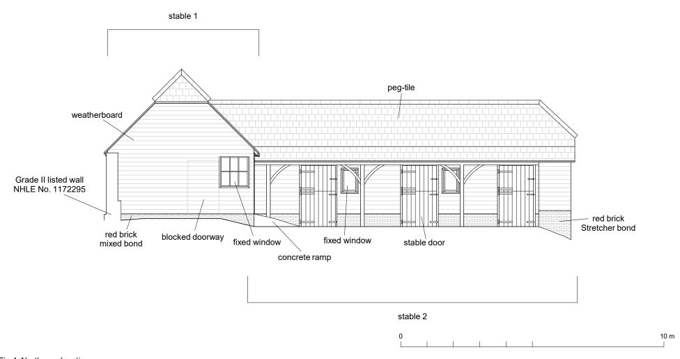
Fig 4 Northern elevation.
