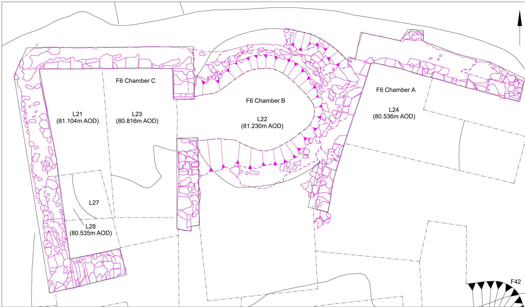
Fig 7 Lime kiln F6 detailed plan.
