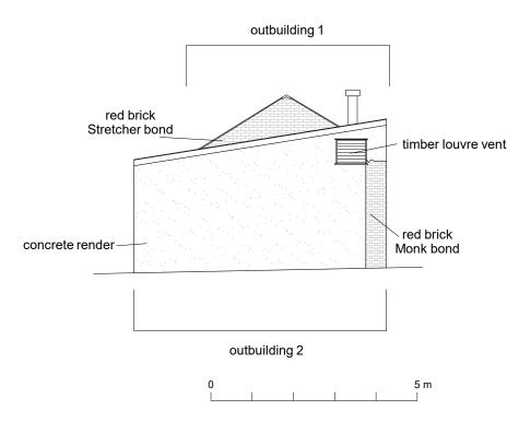
Fig 4 South-east elevation.
