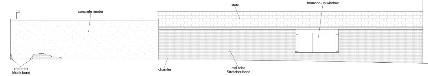
Fig 5 North-east elevation.
