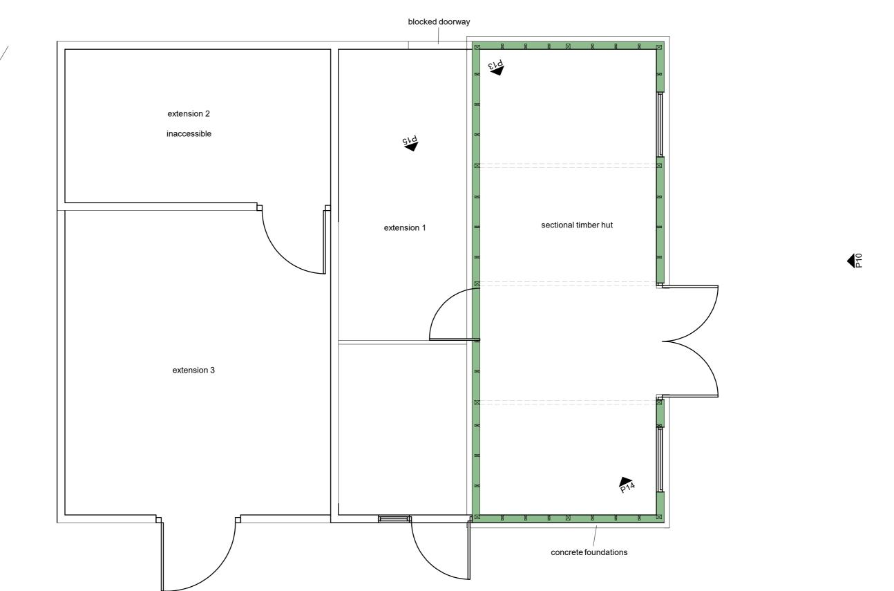
Fig 6 Sectional timber hut floor plan. The original footprint of the hut highlighted in green. Location and direction of photographs reproduced in the text shown.
