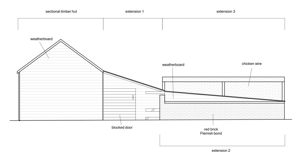
Fig 10 Southern elevation of the sectional timber hut.
