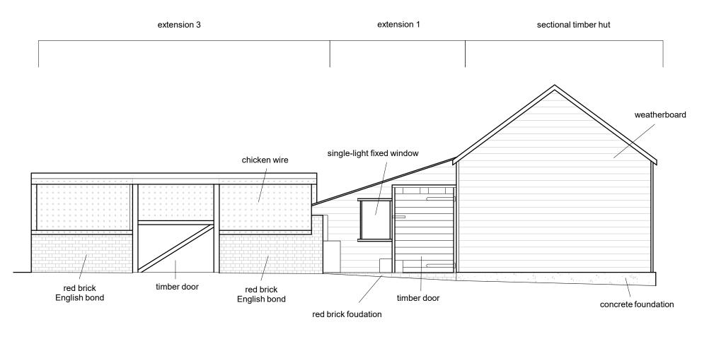
Fig 8 Northern elevation of the sectional timber hut.
