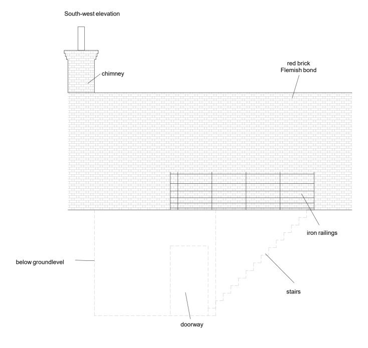
Fig 12 South-west and north-west elevations of boilerhouse.
