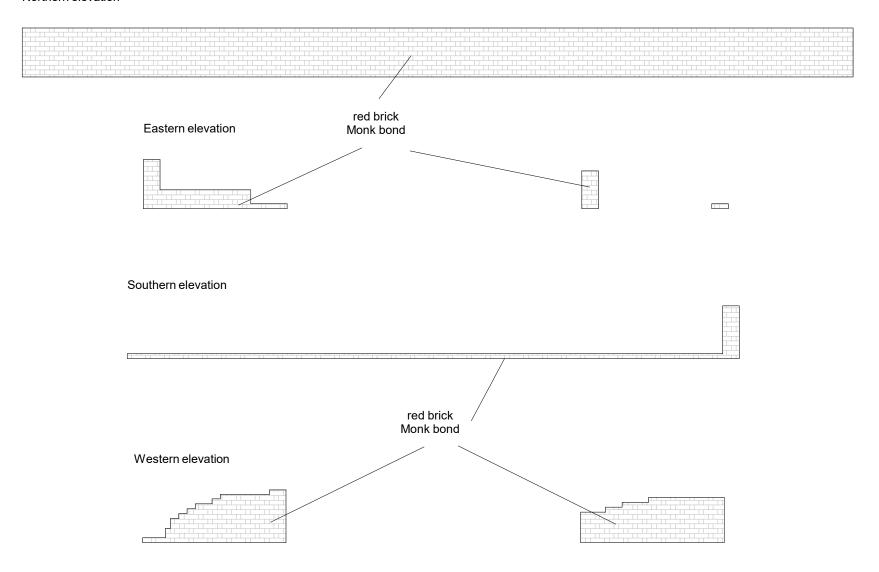
Fig 18 Raised bed elevations.
