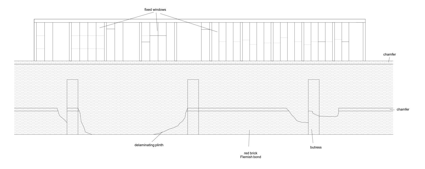
Fig 9 Northern elevation of glasshouse.
