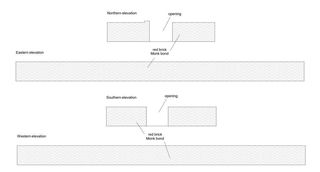
Fig 16 Glasshouse base B elevations.
