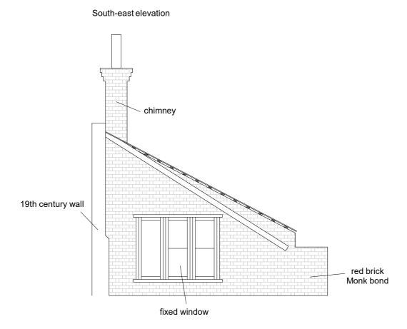
Fig 11 South-east and north-east elevations of boilerhouse.
