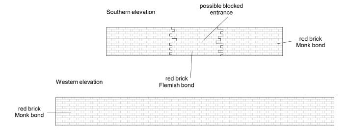
Fig 14 Glasshouse base A elevations.
