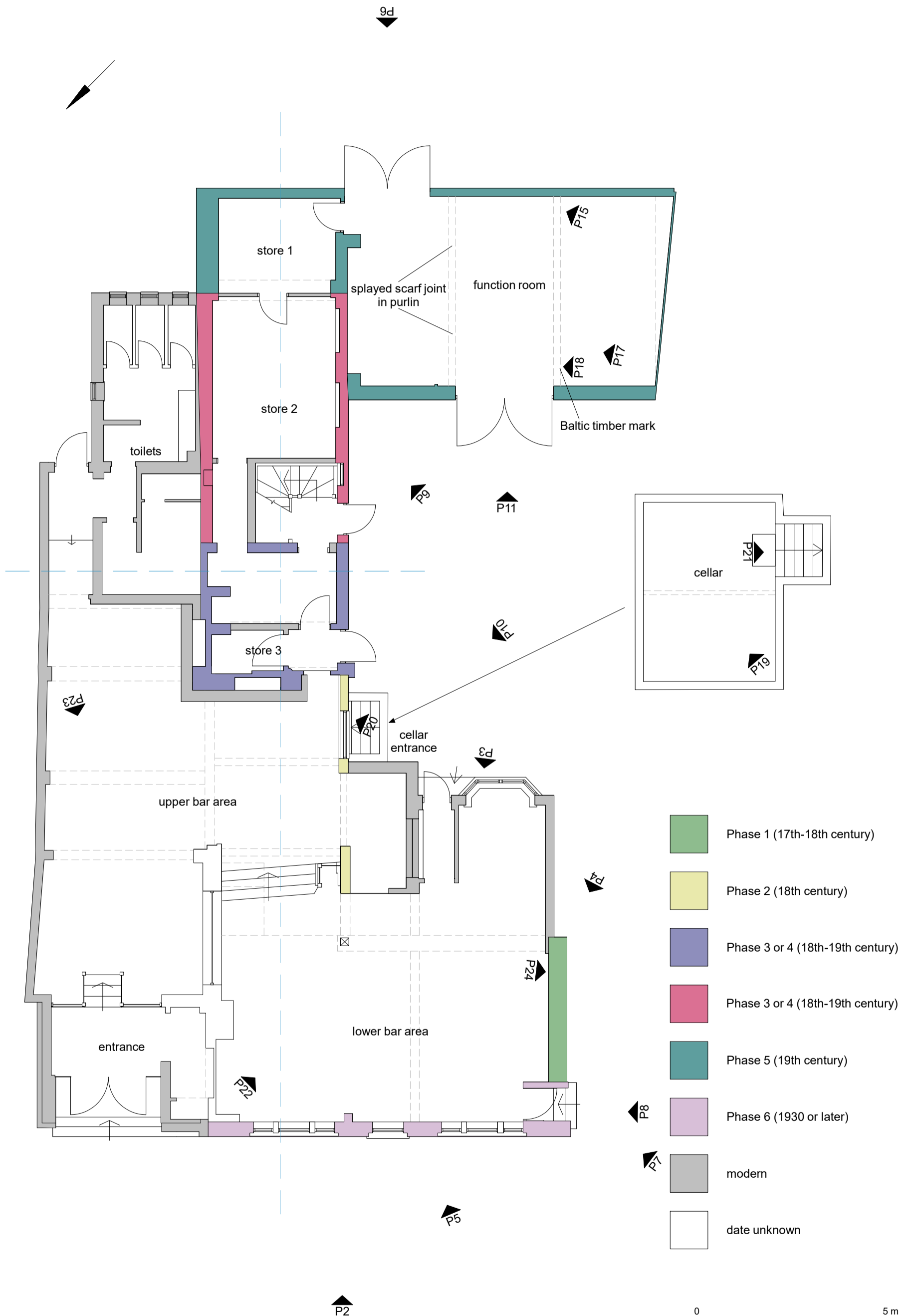
Fig 3 Ground floor plan with cellar plan. Location and direction of photographs reproduced in the text shown. Cross section locations show in blue (Fig 10)
