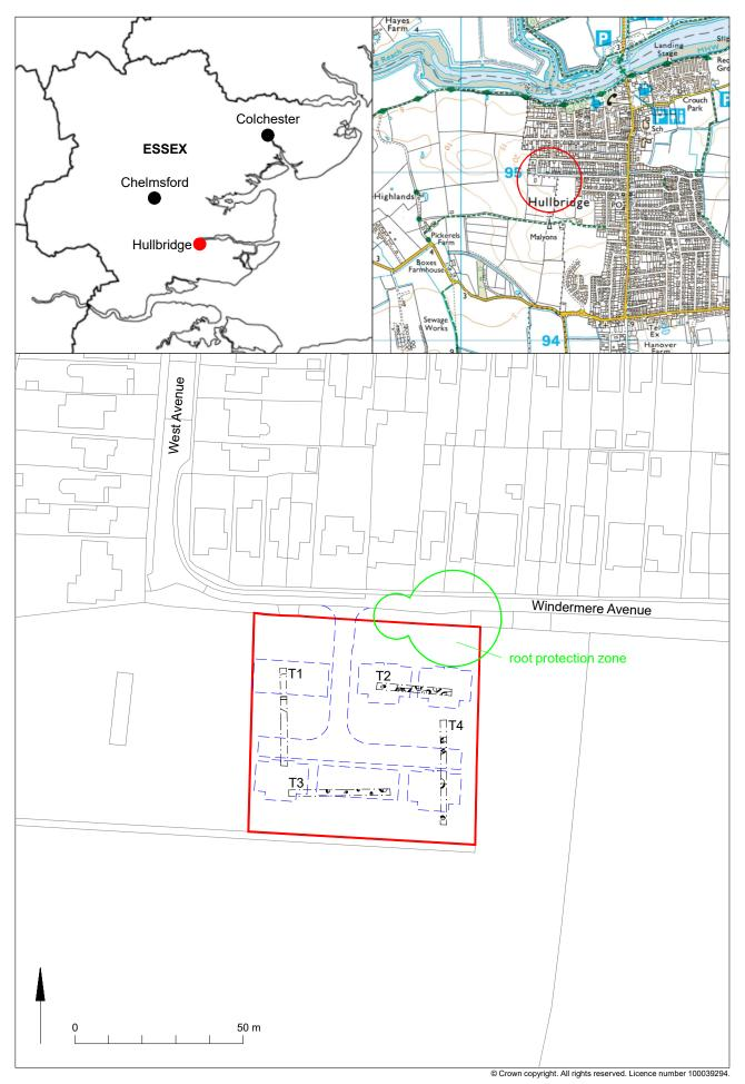
Fig 1 Site location and trench layout in relation to the proposed development (dashed blue).
