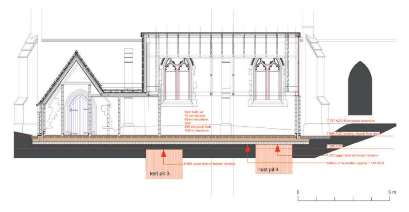
Fig 3 Architectural design showing depth of the proposed flat slab foundation in relation to the evaluation test pits and height of human remains recorded.
