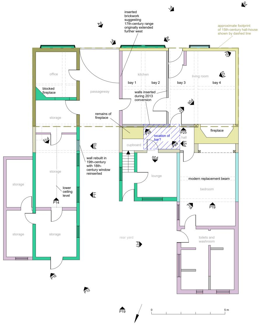
Fig 2 Ground-floor plan of the former Fleece public house, with phasing (derived from listing entry). Location and direction of photographs reproduced in text shown.
