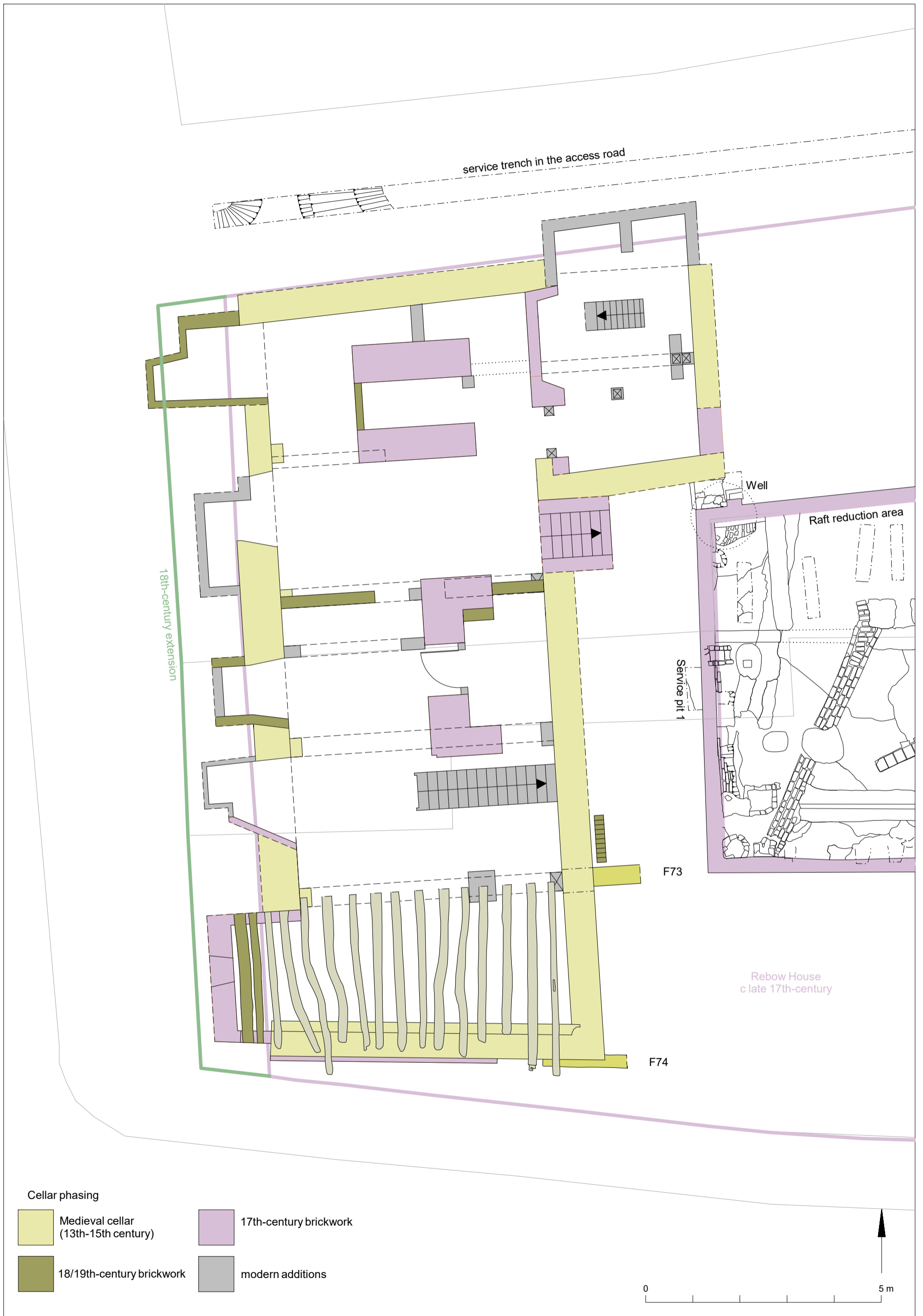
Fig 11 Plan of the medieval cellar plus wall foundations F73 & F74 (see Fig 12 for further details)
