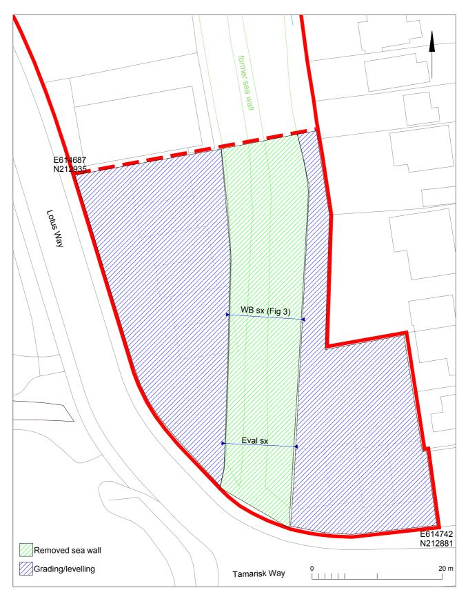
Fig 2 Removal of seawall, grading/levelling results.
