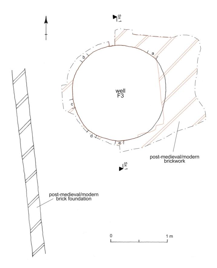
Fig 4 Well (F3): plan. The brick courses in the top of the well and the remains of the brickwork that overlay it are shown in red.
