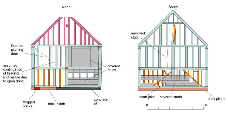
Fig 10 Frame drawing of the north and south walls of the barn, indicating the locations of original, re-used and replacement timbers.
