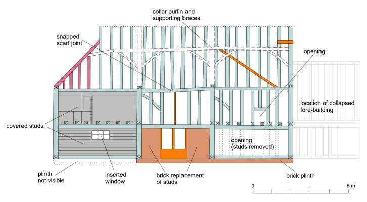
Fig 9 Frame drawing of the east wall of the barn, indicating the locations of original, re-used and replacement timbers.
