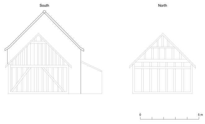
Fig 7 Frame drawings of the fore-building prior to its demolition (taken from pre-existing architects drawings).
