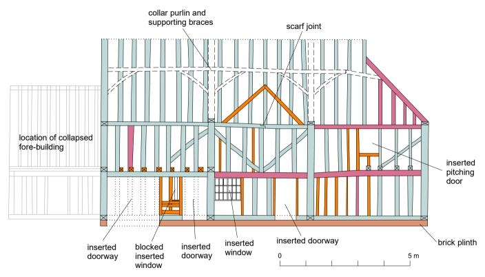
Fig 8 Frame drawing of the west wall of the barn, indicating the locations of original, re-used and replacement timbers.
