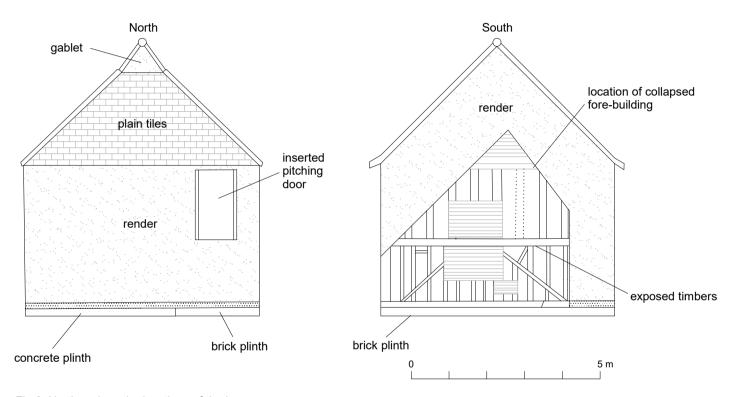
Fig 6 North and south elevations of the barn.
