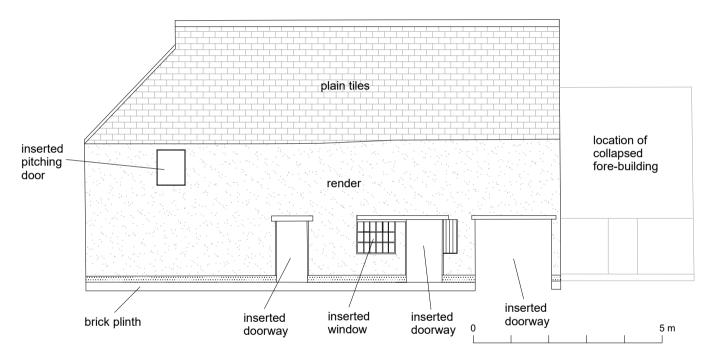
Fig 5 West elevation of the barn.
