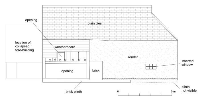
Fig 4 East elevation of the barn.
