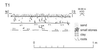
Fig 3 Representative trench section.
