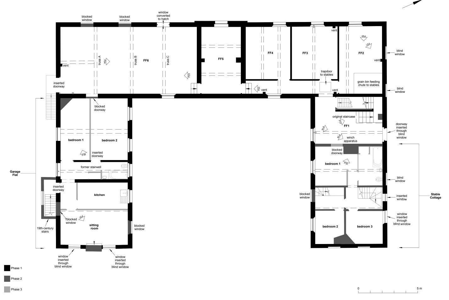
Fig 4 Structure 1/2, 18th-century stable block first floor plan, showing the location and orientation of photographs included in this report.
