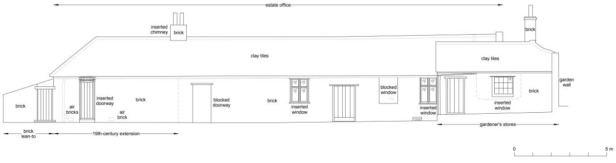
Fig 14 Structures 3 & 3a, 18th-century estate office and gardener's stores north-west elevation.
