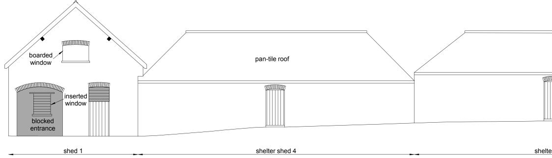
Fig 10 Kitchen Farm, north-west elevation with alterations shaded grey.
