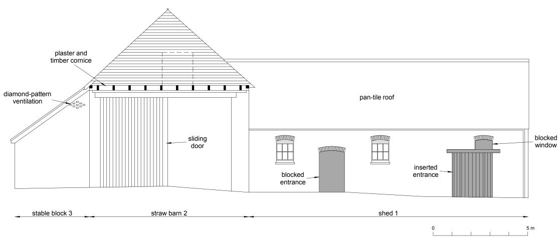
Fig 7 Kitchen Farm, north-east elevation with alterations shaded grey.
