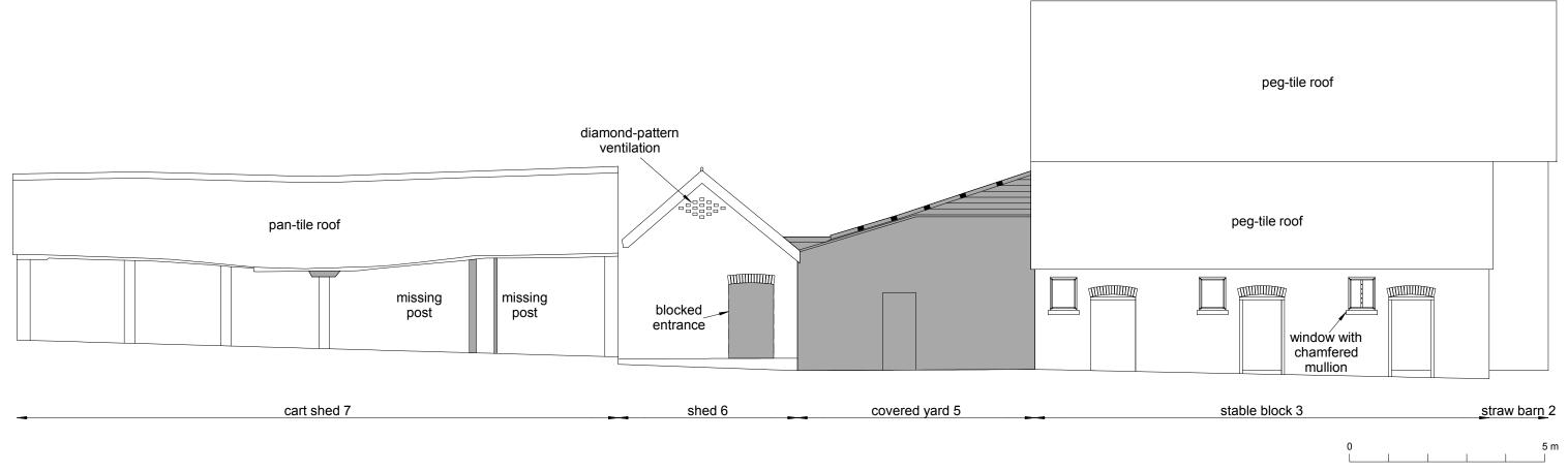
Fig 8 Kitchen Farm, south-east elevation with alterations shaded grey.
