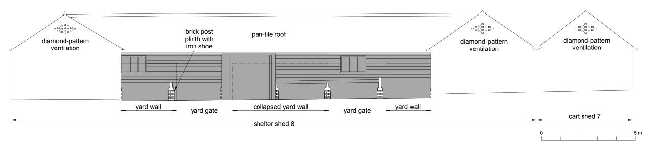
Fig 9 Kitchen Farm, south-west elevation with alterations shaded grey.
