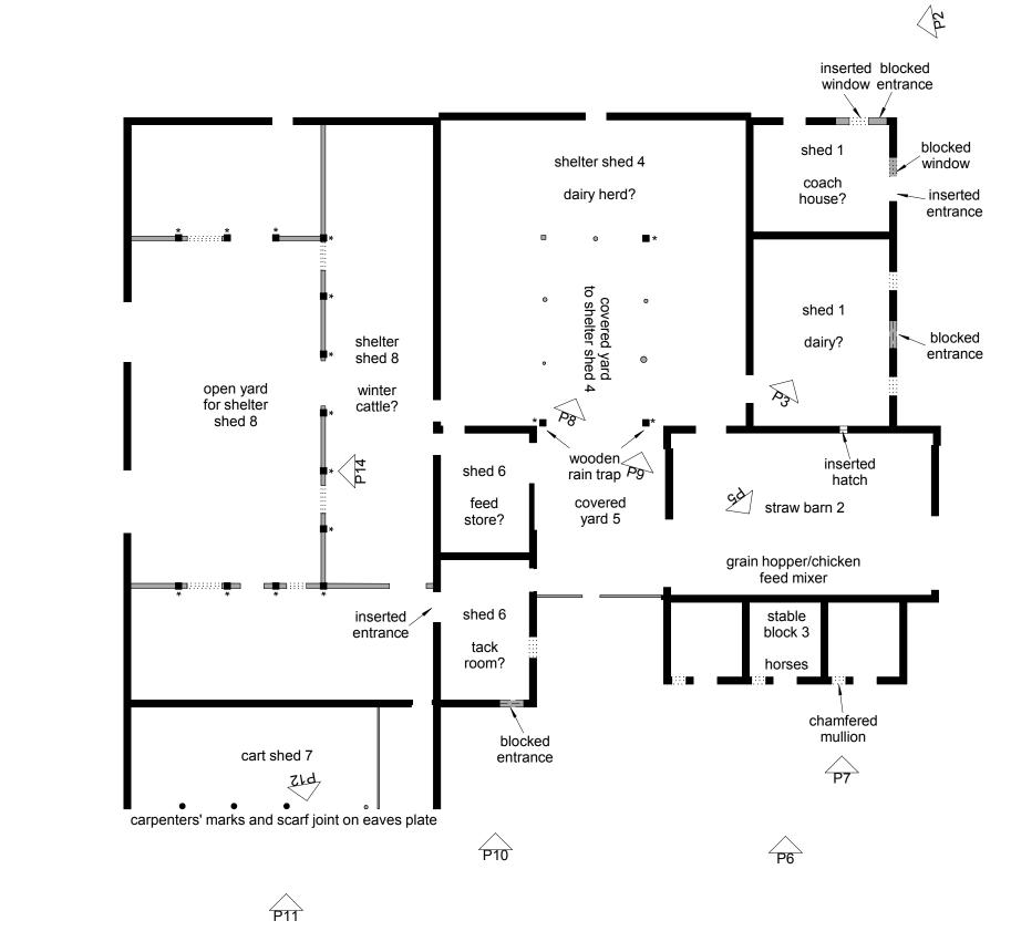
Fig 6 Kitchen Farm floor plan showing location and orientation of photographs included in the report, with alterations shaded grey.
