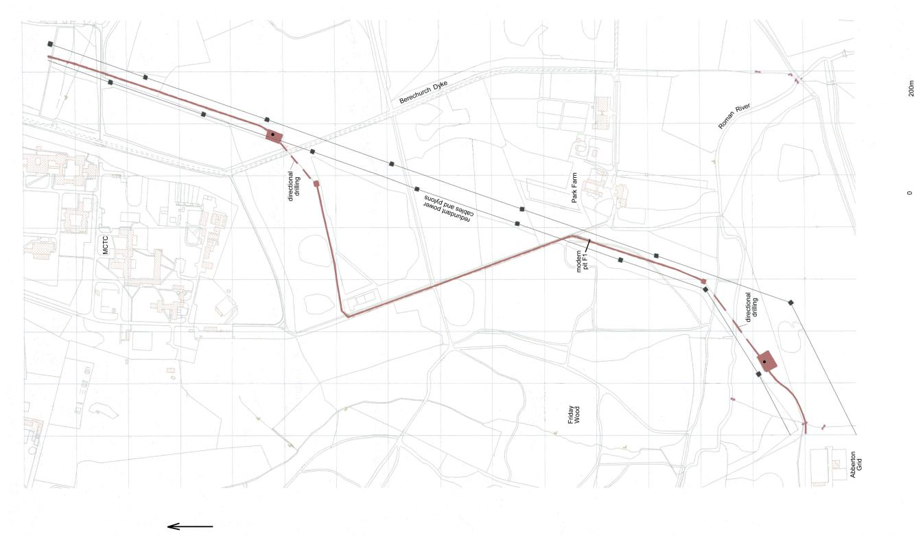
Fig 1 Site location plan, showing the course of the cable trench.
