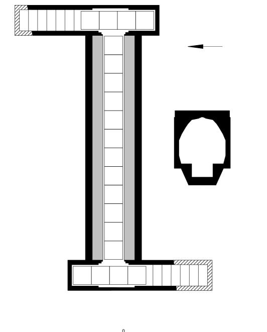
Fig 10 Development Area 7: air-raid shelter WBF82 - plan and cross-section.
