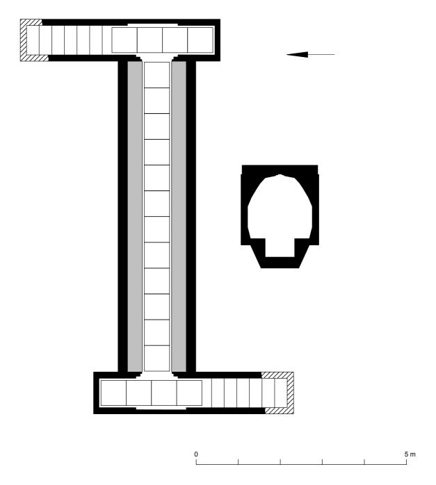
Fig 14 Development Area 7: air-raid shelter WBF103 - plan and cross-section.
