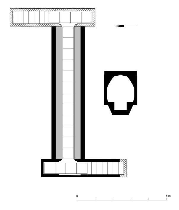
Fig 13 Development Area 7: air-raid shelter WBF85 - plan and cross-section.
