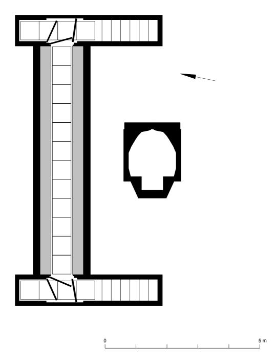
Fig 15 Development Area 8: air-raid shelter WBF102 - plan and cross-section.
