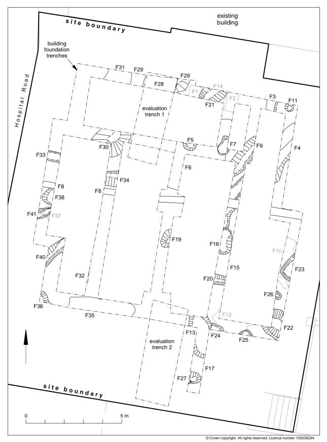
Fig 2 Plan of site, showing trenches and features (grey features are earlier).
