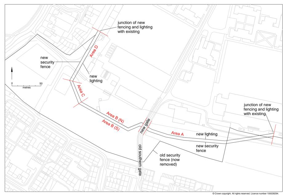
Fig 2 Plan of the new security fencing and lighting erected on the southern side of the Kirkee McMunn barracks.
