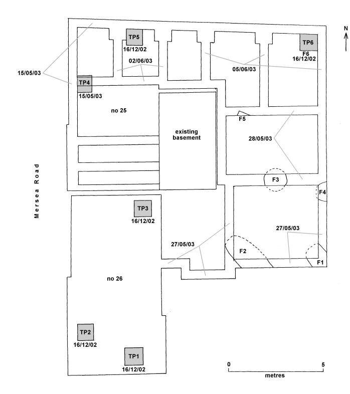
Fig 2 New foundation trenches: plan, showing the areas monitored and the dates on which the monitoring took place - scale 1:100.
