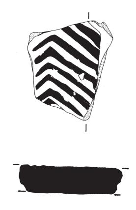
Fig 9 Tile with relief-pattern keying (die 42 or similar) from F6, scale 1:1.
