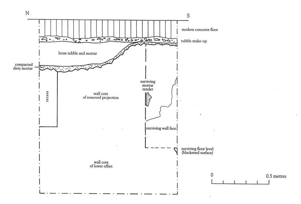
Jacklins, High Street, Colchester, 1997: pile cap 1 - medieval wall (F1), section
