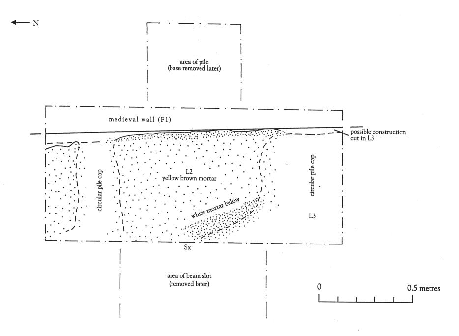
Jacklins, High Street, Colchester, 1997: pile cap 3, plan
